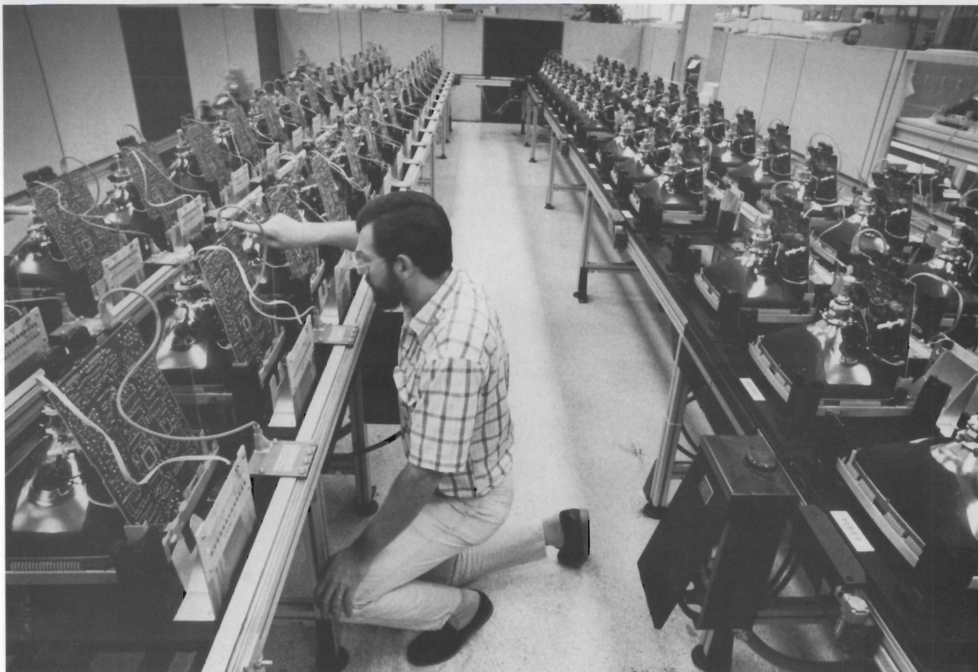
Video cameras mounted near the floor monitor information on the CRT screens as the terminals wind their way through a two- to four-hour self-testing area. John Spaeth, test technician, gives the made-in-America terminal line an added visual check.
