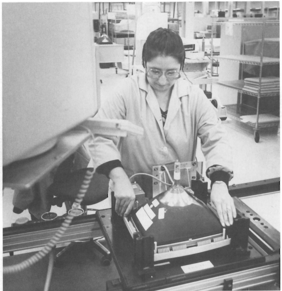
Stella Hernandez places the cathode ray tube face down onto the terminal’s plastic frame. Top-down assembly means workers never have to turn the terminals around.
