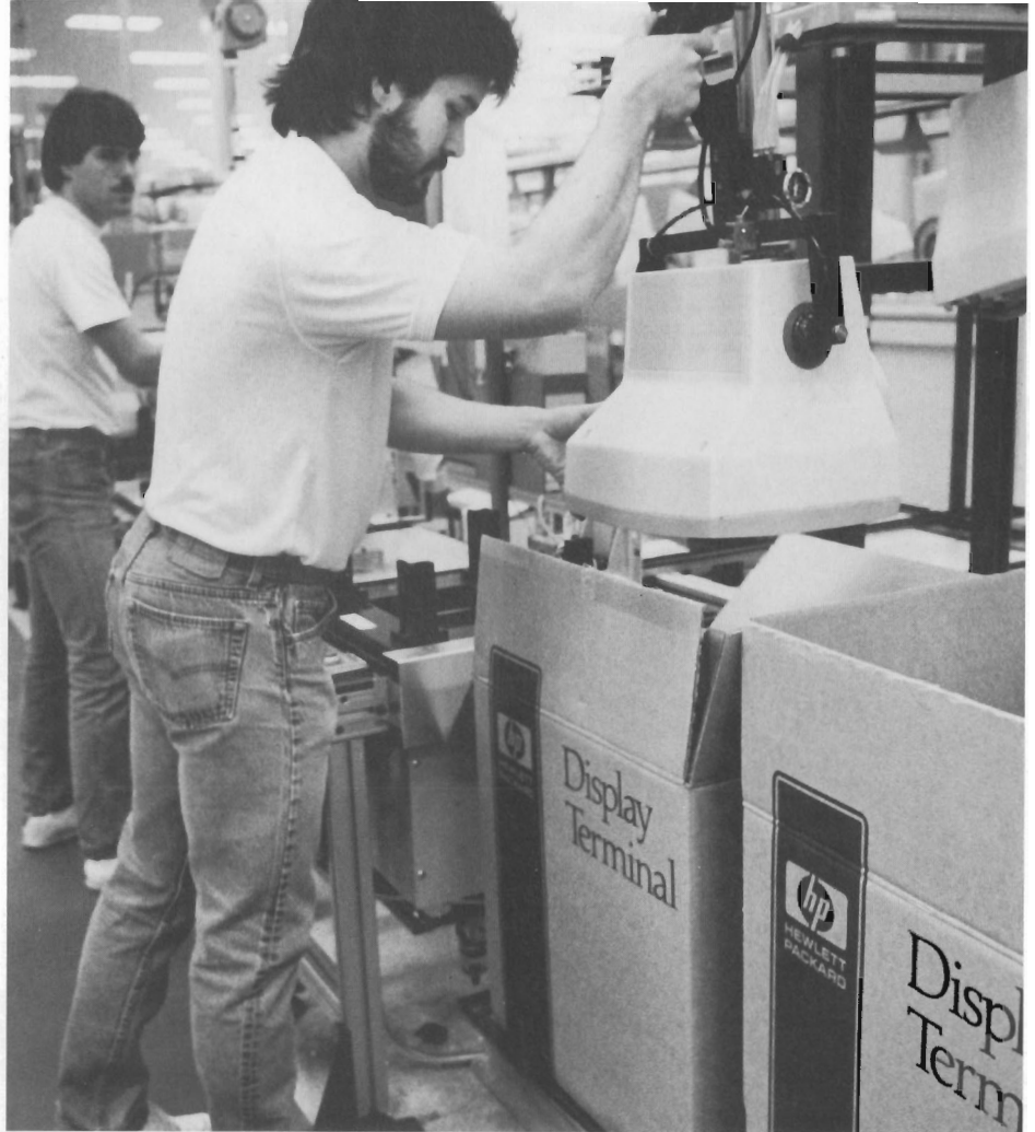
Ben Seligson uses a pneumatic arm to insert a completely built HP series 700 computer terminal in its shipping box at the end of the manufacturing line.
