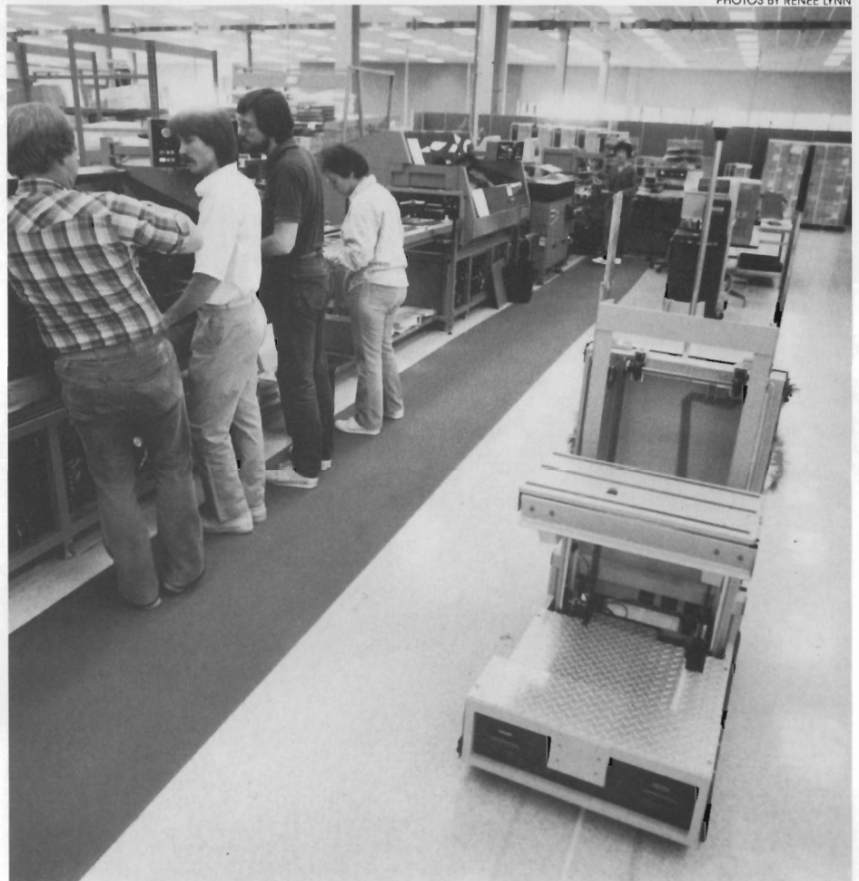
An automated vehicle, which follows an electronic path in the manufacturing floor, carries printed circuit boards from one workstation to another.
